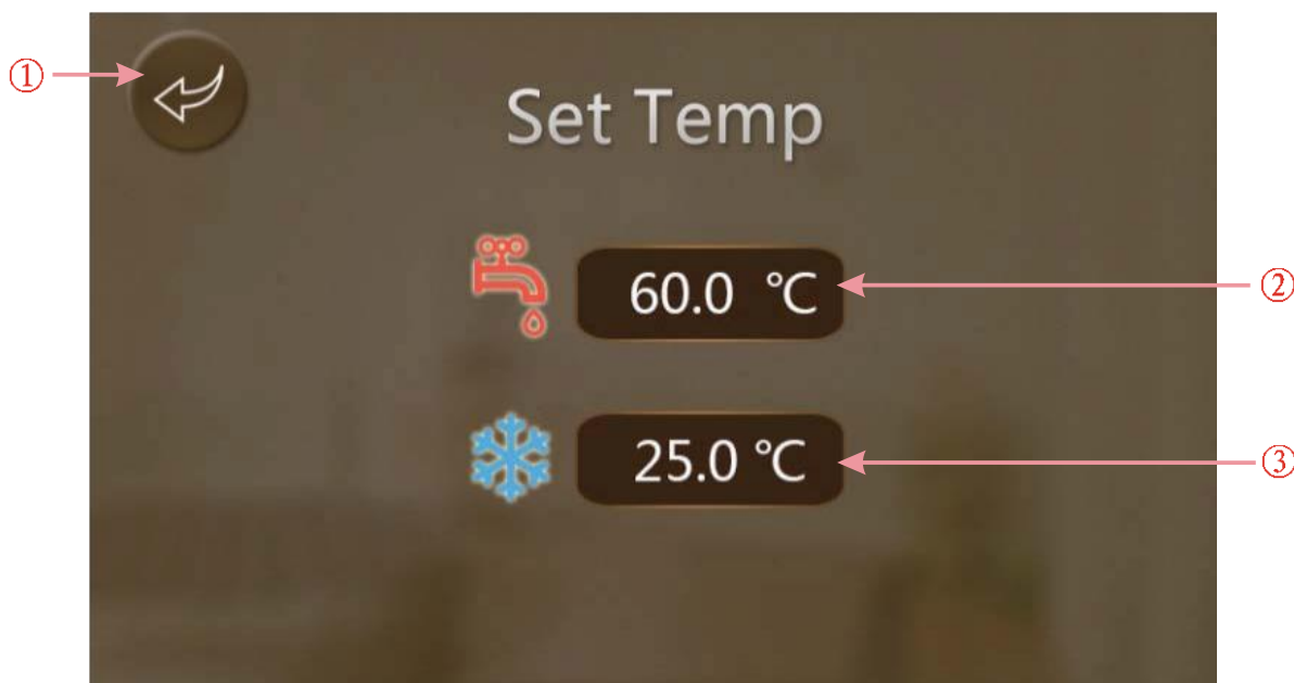
Tribunewater heating + jahutuse seadete seadistamine
